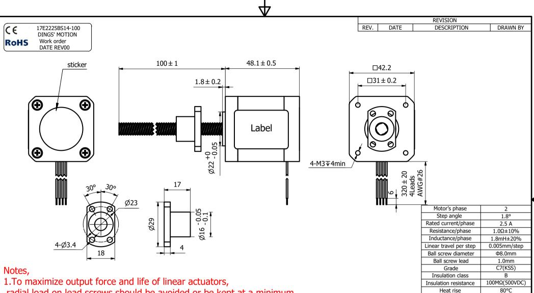
radial load on lead screws should be avoided or be kept at a minimum.
