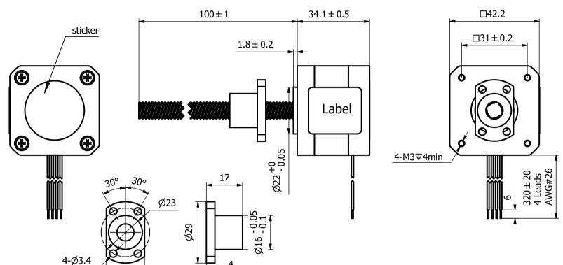
Motor's phase Step angle 1.8° Rated current/phase 1.0 A Resistance/phase 3.8Ω±10% Inductance/phase 5.0mH±20% 0.005mm/step Linear travel per step Ball screw diameter Ф8.0mm Ball screw lead 1.0mm C7(KSS) Grade Insulation class 100MΩ(500VDC) Insulation resistance 80°C Heat rise 0.25 kg Motor weight
