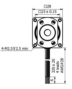
Motor's phase 2 Step angle 1.8° Rated current/phase 1.0 A 2.1Ω±10% Resistance/phase Inductance/phase 1.5 mH±20% 0.01mm/step Linear travel per step Ball screw diameter Ф6.0mm 2.0mm Ball screw lead C7(KSS) Grade Insulation class 100MΩ(500VDC) Insulation resistance Heat rise 80°C 0.12 kg Motor weight
