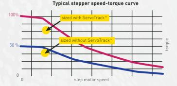
ServoTrack™ control is hardware based for real-time response. It continually monitors the relationship between the rotor and stator at nano-second intervals, and will not allow that relationship to exceed the point where motor synchronization is lost.
