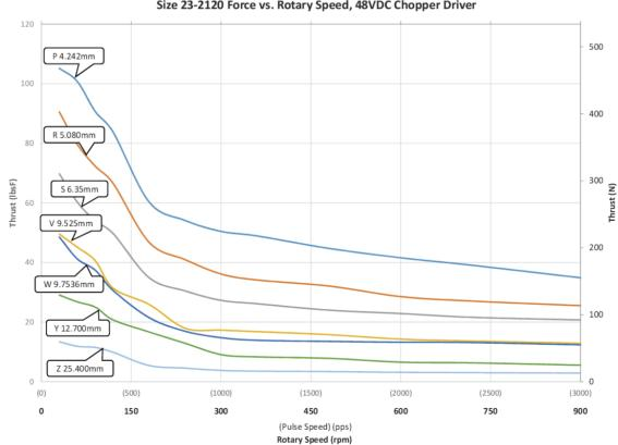
Size 23-2120 Force vs. Rotary Speed, 48VDC Chopper Driver
